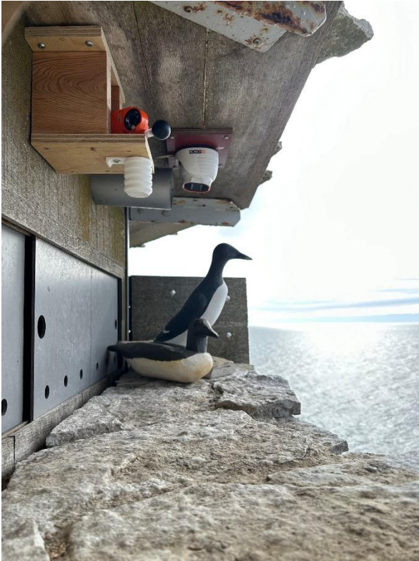
Fig. 5. The 3D printed radiation screen: white cylinder attached to the wooden box. Two dummy guillemots on the ledge. (Photo: David Stone)
