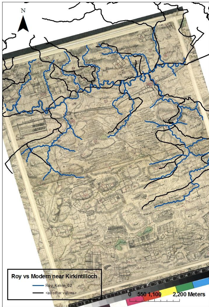
Fig. 3. Comparison of the River Kelvin system near Kirkintilloch as portrayed by the Roy Map (1752-1755) and the 2010 Ordnance Survey reported as "<all other values>" (map provided by the British Library, 2013).
